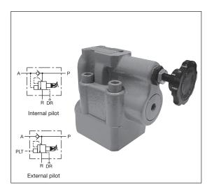
This type of valve consists of a balance piston type unloading valve and a check valve assembled in one housing and is mainly used in accumulator circuits and circuits in which two levels of pressure (low-pressure large-volume circuit and high-pressure small-volume circuit) are handled.
